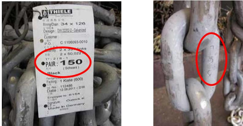
c) The ends of chain pairs are marked in the same color.
