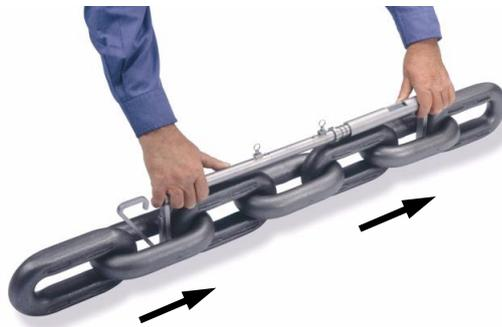
In addition to measurements with the chain gauge, suitable chain pieces (7 links, no fitting chains) can also be sent to THIELE for testing. For the test pieces, it shall be ensured that the specimens have the same running time as the rest of the chain.
